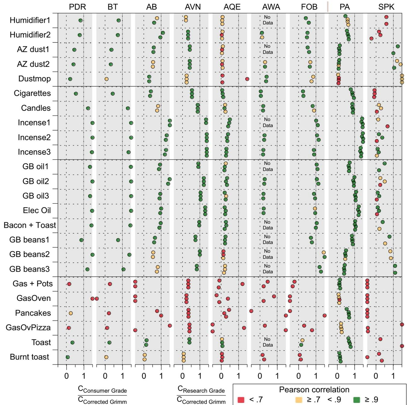
**FIGURE 7** Regression coefficients and correlation statistics for baseline-subtracted, time-resolved data from tested devices related to density-adjusted data from Grimm Mini Wide-Range Aerosol Spectrometer. For PA, the 4 data points come from 2 devices which each had 2 sensors. Ratios of 1.5 or greater plotted at 1.5. Ratios below zero indicate inaccurate readings by consumer monitors
