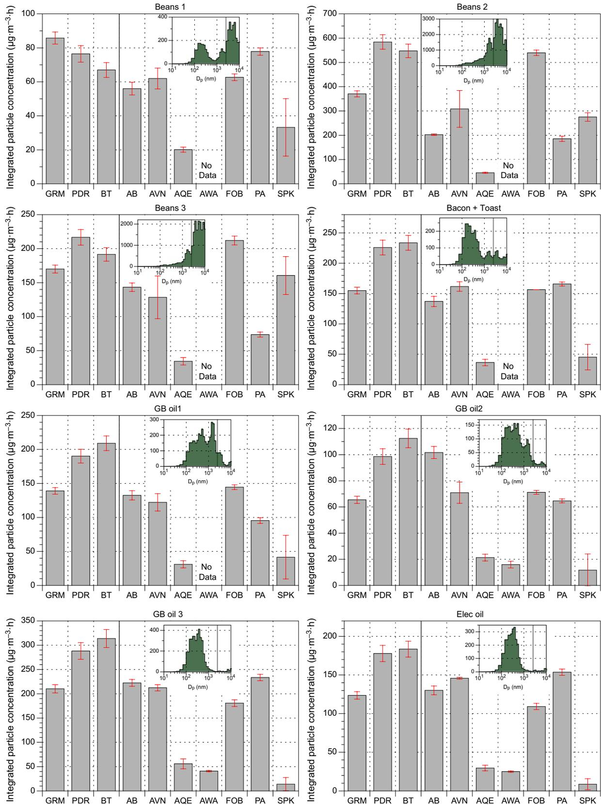
**FIGURE 5** Baseline-subtracted, time-integrated particle concentrations for frying or heating oils. The Grimm Mini Wide-Range Aerosol Spectrometer (GRM) is the estimated true mass concentration. Inset panels show the distribution of mass by particle size ( $dM/d\log D_p$ ) at the peak
