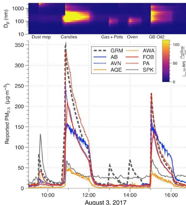
**FIGURE 2** Example results from 5 source experiments. For devices that sampled more frequently than each minute, data have been averaged for 1-min resolution. The top portion of plot shows the distribution of mass by particle size. Refer to Table 2 for monitor abbreviations
