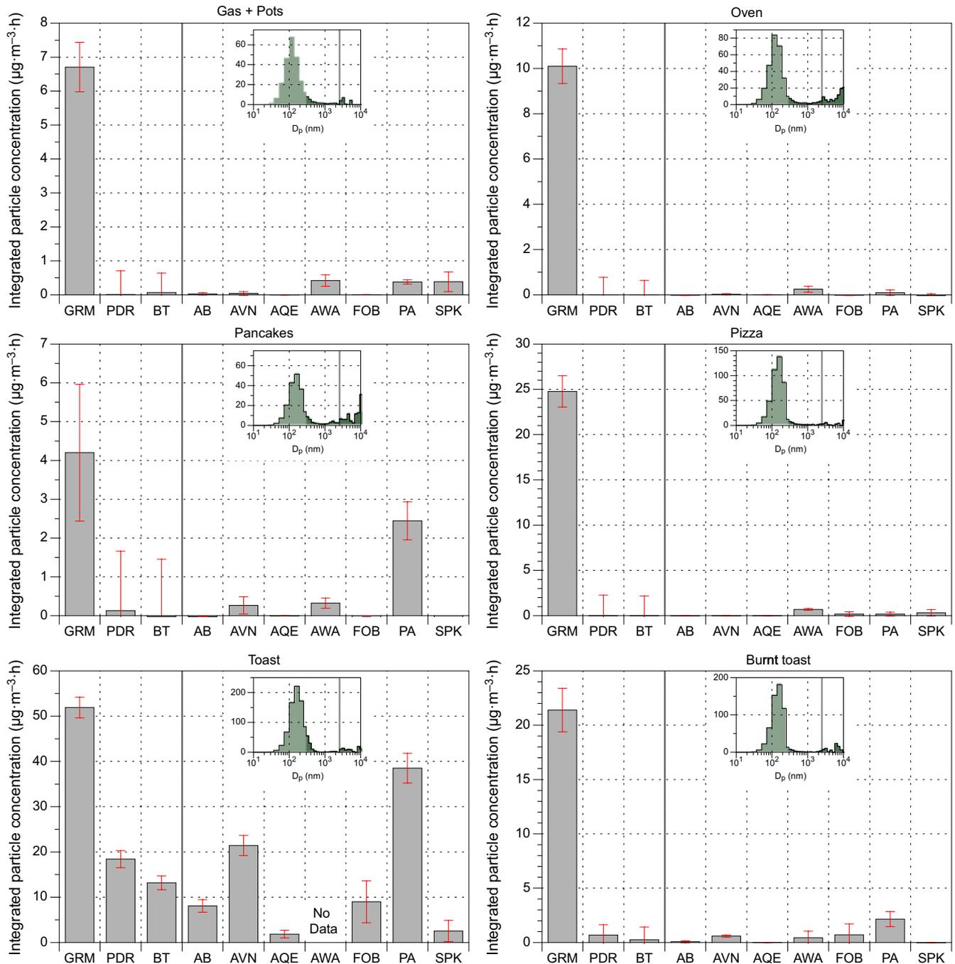
**FIGURE 6** Baseline-subtracted, time-integrated particle concentrations for cooking sources that generated substantial quantities of ultrafine particles but relatively little mass. The Grimm Mini Wide-Range Aerosol Spectrometer (GRM) is the estimated true mass concentration. Inset panels show the distribution of mass by particle size ( $dM/d\log D_p$ ) at the peak
