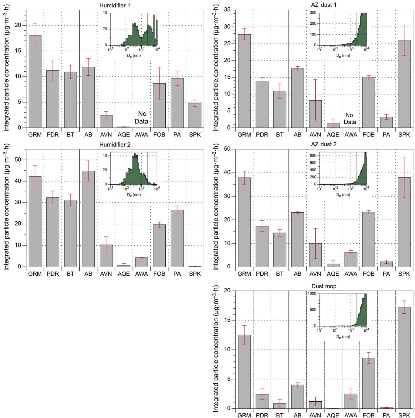
**FIGURE 3** Baseline-subtracted, time-integrated particle concentrations for ultrasonic humidifier without filter and dust sources. The Grimm Mini Wide-Range Aerosol Spectrometer (GRM) is the estimated true mass concentration. Inset panels show the distribution of mass by particle size ( $dM/d\log D_p$ ) at the peak
