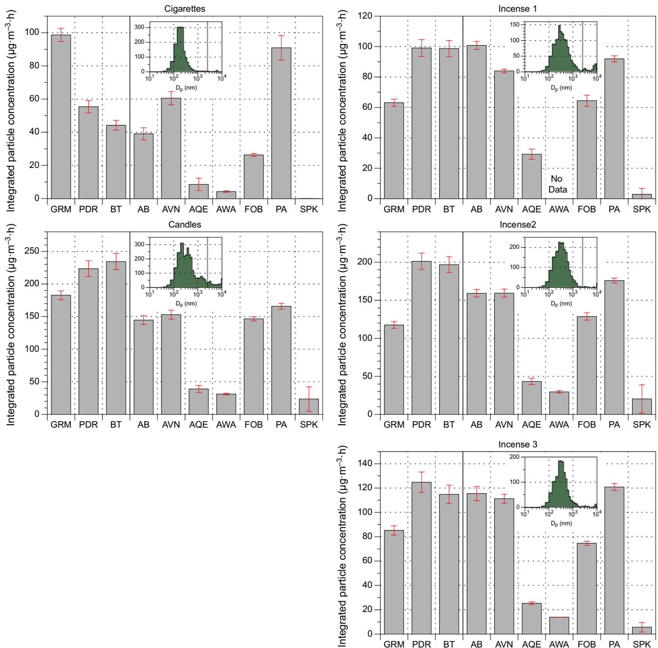
**FIGURE 4** Baseline-subtracted, time-integrated particle concentrations for recreational combustion sources. The Grimm Mini Wide-Range Aerosol Spectrometer (GRM) is the estimated true mass concentration. Inset panels show the distribution of mass by particle size ( $dM/d\log D_p$ ) at the peak
