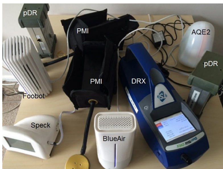
Fig. 1. Experimental setup of a residential PM_{2.5} monitoring station.
